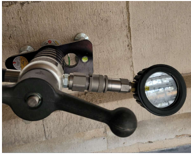
Pull Testing PPE Eyebolts at LSO
